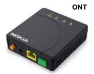
This device is required to connect to the fibre network. This ONT is owned by IFSNZ and is not serviceable by you or your ISP and must remain within the property.
